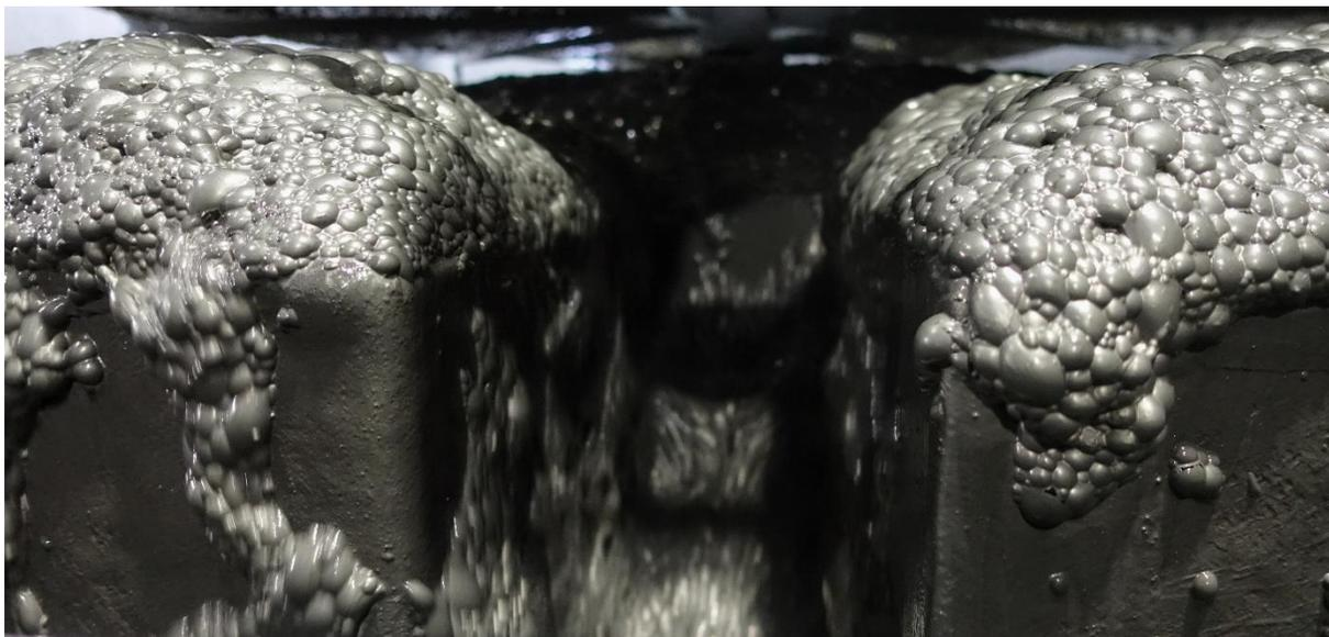
7. To produce the pure metal, further treatments such as melting furnaces are needed. Melting can further separate the recovered minerals to produce pure metal for use in cell phones, cars, plumbing, electricity, and many other things we use daily.
