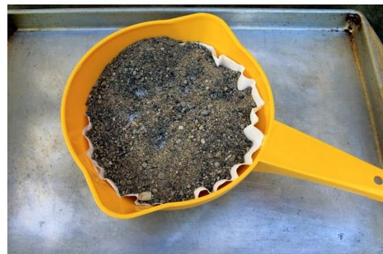
The cookie sheet or baking pan represents the liquid collection system. Very slowly sprinkle a liter of water over the top of the “low-grade ore” for about 5 -10 minutes in order to dissolve the salt from the low-grade ore body. Capture all the liquid from this leaching of the low-grade ore heap in the cookie sheet or baking pan.
