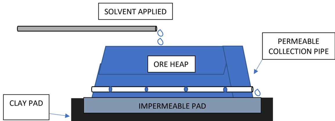
An example of this process is the recovery of copper from a low-grade copper oxide ore with the use of dilute sulfuric acid. The resulting copper sulfate solution is transferred from the collection system and the copper is recovered by electrolysis (separation of charges) or chemical replacement reactions using
