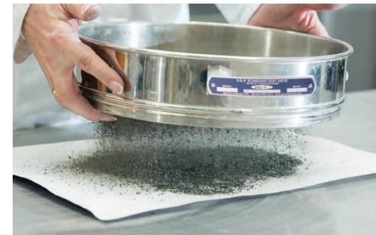
A technician using a screen to sort rock particles.
