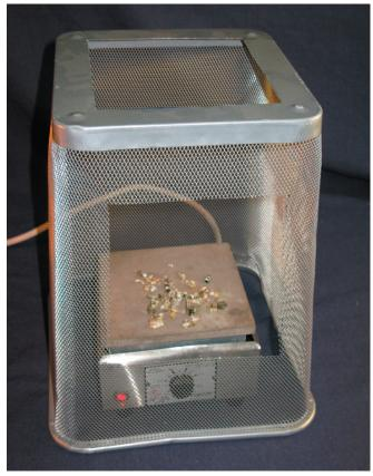
boiling blows the kernel open. Vermiculite, like all micas, is a sheet silicate. When heated, water between the layers of the vermiculite expands and pushes the sheets apart (to the point where the water vapor can escape).
