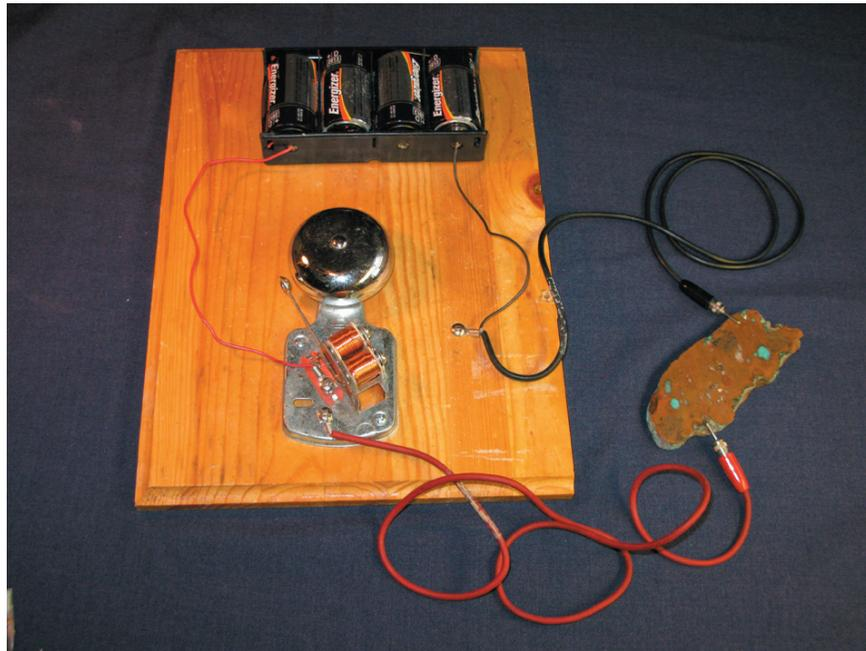
Procedure description: Students bring both of the leads of a conductivity tester into contact with a specimen to test if it will pass electricity.
